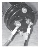
Switch to Battery Fuse Connections
